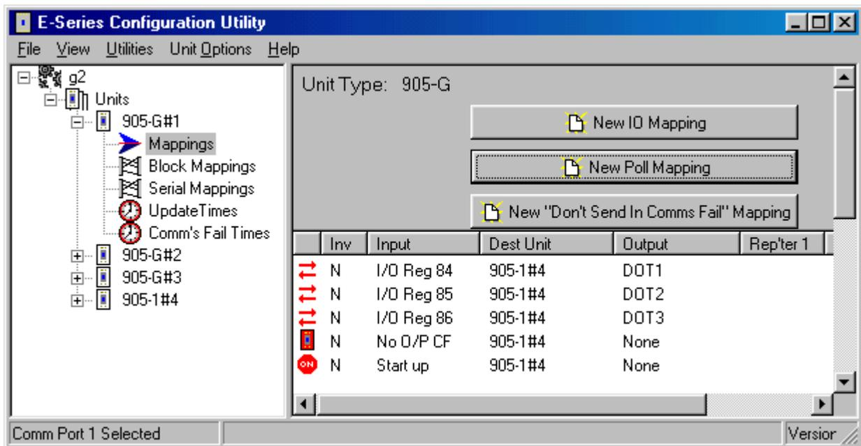
To configure this special mapping, select the “New Don’t Send in Comms Fail Mapping” box. You will be asked to select which remote module this function applies to. You can enter more than one of these mappings if there are more than one modules.
