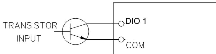
All eight of the 105G DIO terminals may also be used as discrete outputs. The digital outputs are transistor switched DC signals, FET output to common rated at 30VDC 500 mA.
