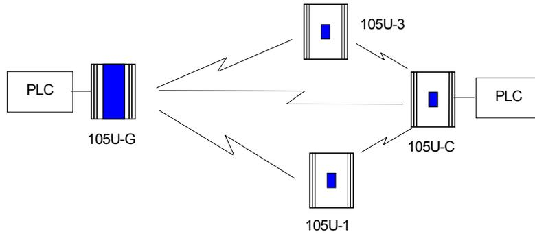
105G modules can transmit to 105G modules as well as other 105G modules. There can be multiple 105G and 105C modules in a network - as well as 105U I/O. Because the 105U protocol is peer-to-peer, there are few constraints on communications between multiple 105U modules.
