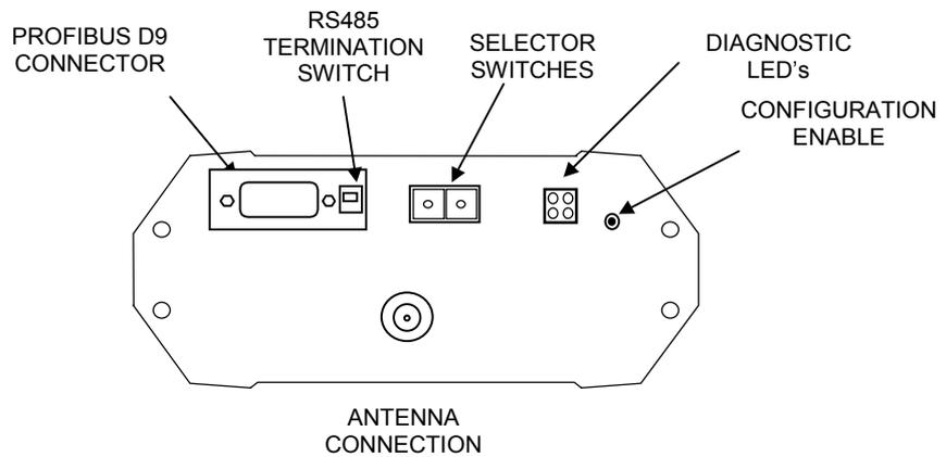
Note: The rotary selector dial on the end plate should be set to zero. If it is set to a non-zero position, the user-configured Profibus Slave address will be over-written by the selection.
