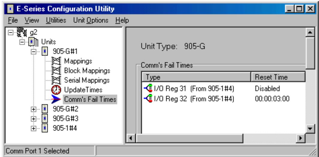
The default value for the comms-fail time is “disabled” or zero. To enter a time, select the I/O register from the list. The comms-fail time should be greater than the update time of the remote input.
