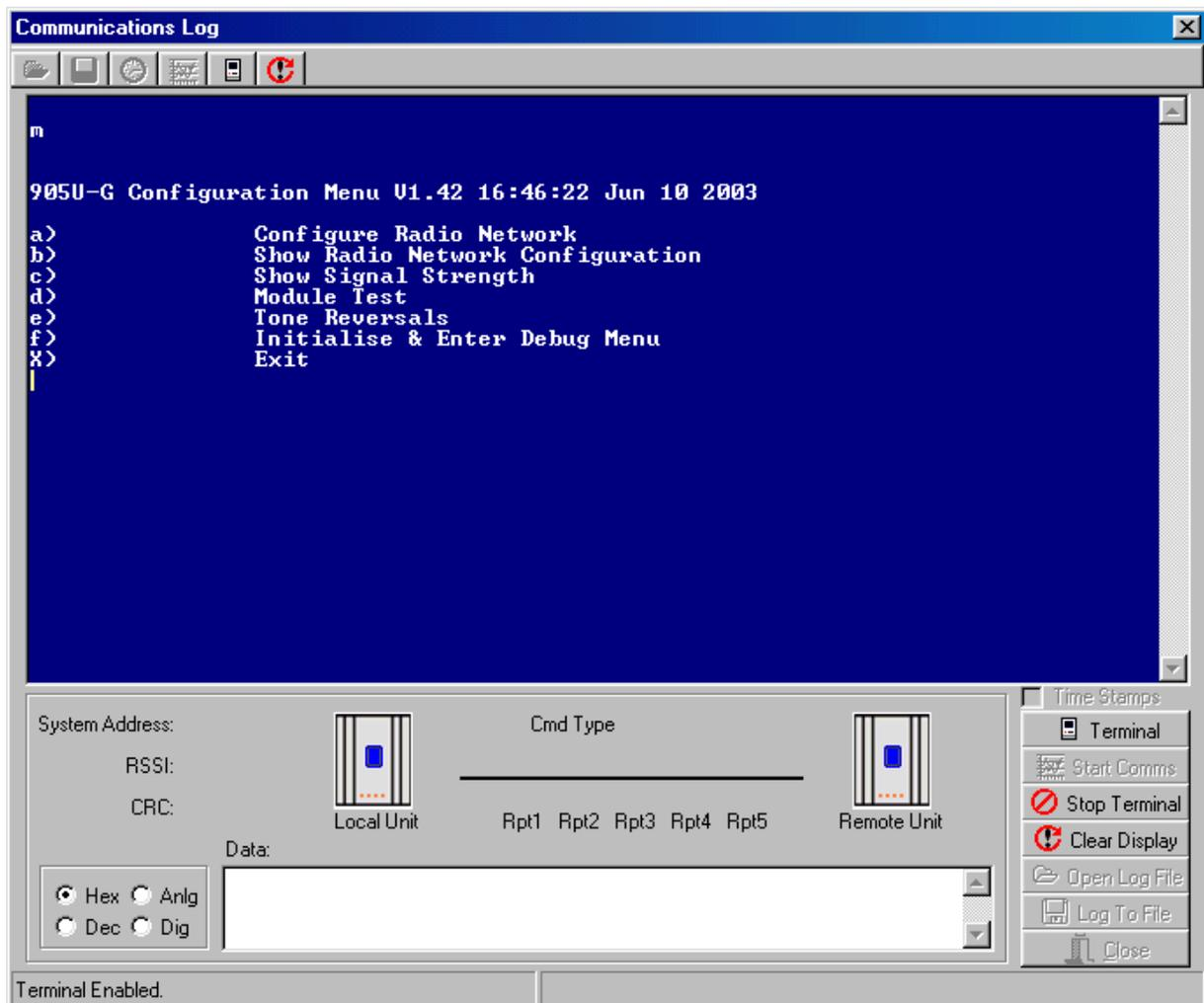
**Note:** Options a), b), d) and f) are used in factory test and should not be selected.
