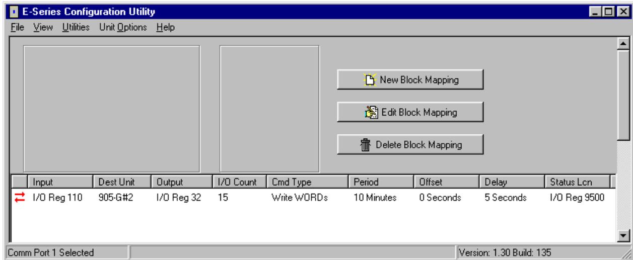
In the above example, the status register for the block mapping has been automatically assigned to register 9500.
