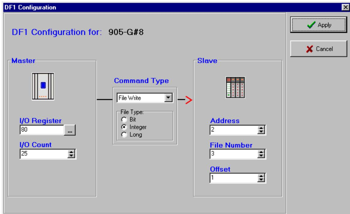
The entry under “I/O Register” is the first I/O register in the 105G to be transferred - the “I/O count” is the number of registers to be transferred.
