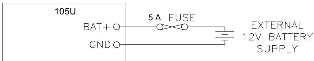
Upon failure of the normal supply, the module may continue to operate for several hours from a backup battery. The battery charger is rated at 1.5A and is designed for sealed or vented lead acid batteries between 5 and 24 amp hours - **other types of batteries should not be used**.
