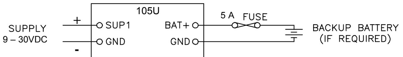
The module may also be powered from an external 11 - 15 VDC battery supply without the need for a "normal" supply connected to "SUP1". This external battery supply is connected to "BAT+" and "GND" terminals. The positive lead of the external supply should be protected by a 5A fuse.
