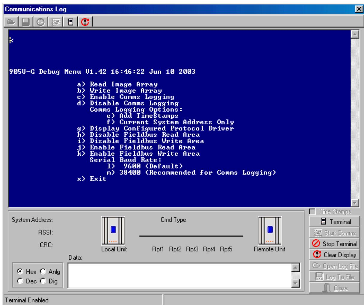
The Debug Menu allows the I/O Database to be viewed and modified to confirm the operation of the radio network. These options may be used to check operation of outputs at remote sites, and to check the values of inputs reported from remote sites.
