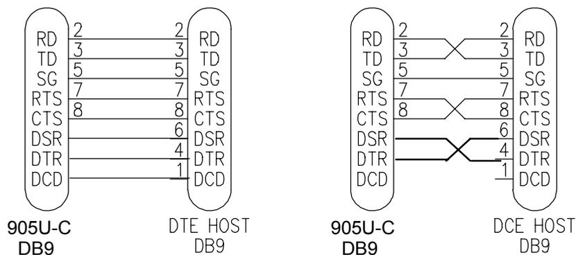
Hardware handshaking using the CTS/RTS lines is provided, and are under the control of the Host Comms Driver. Example cable drawings for connection to a DTE host (a PC) or another DCE host are detailed above.
