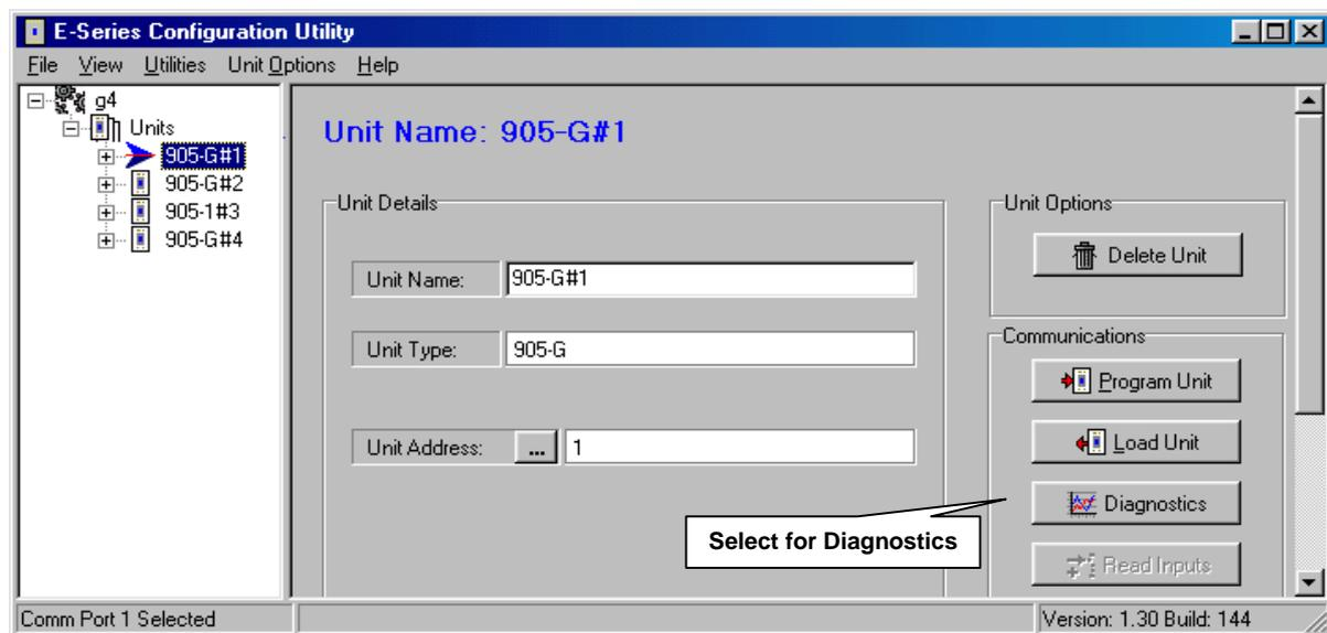
A “Terminal” screen will appear. With this screen, you can enter “off-line” or “on-line” diagnostics. You will need to connect the PC to the 105G using the RS232 configuration cable.
