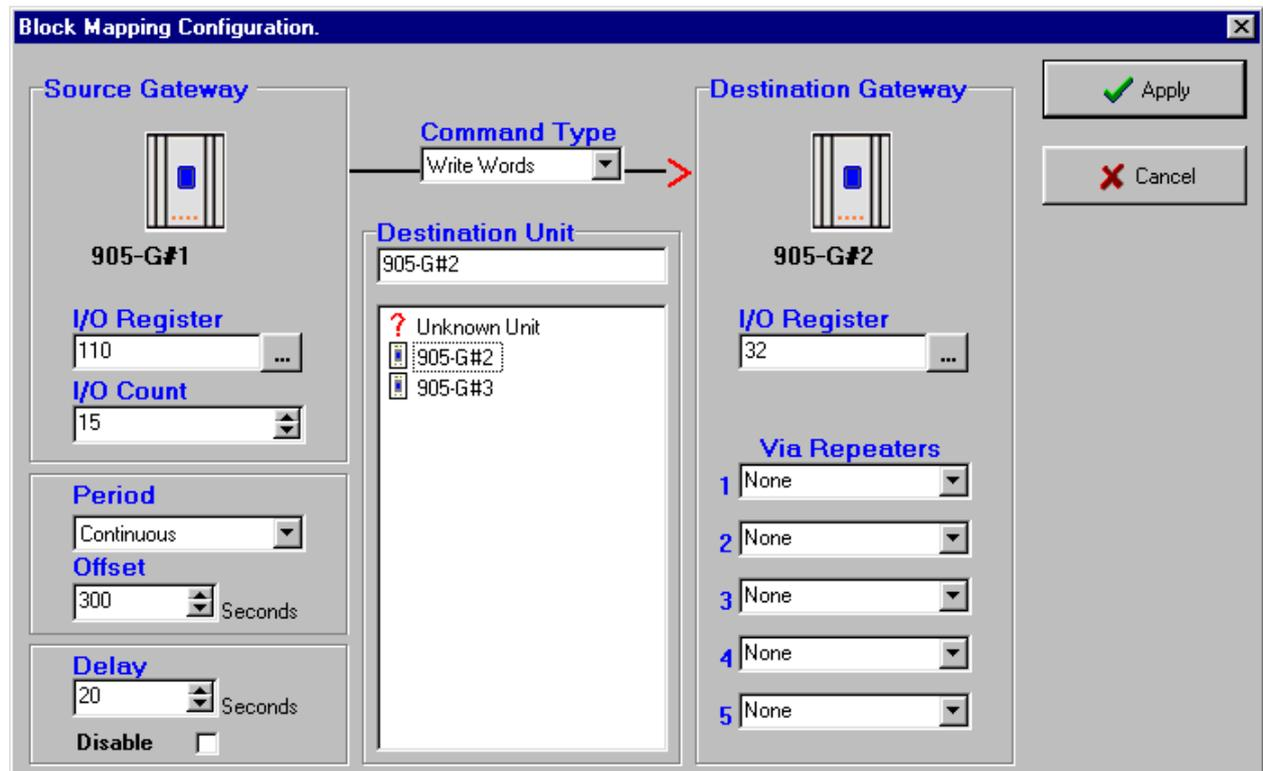
If a value in the block changes by more than the sensitivity amount, then the block message will be sent. The sensitivity values are set under the “Sensitivity” option as per section 4.5.
