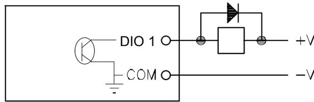
The output circuit is connected to the appropriate "DIO" terminal. Each digital output circuit includes a LED indicator which is lit when the digital output is active.
