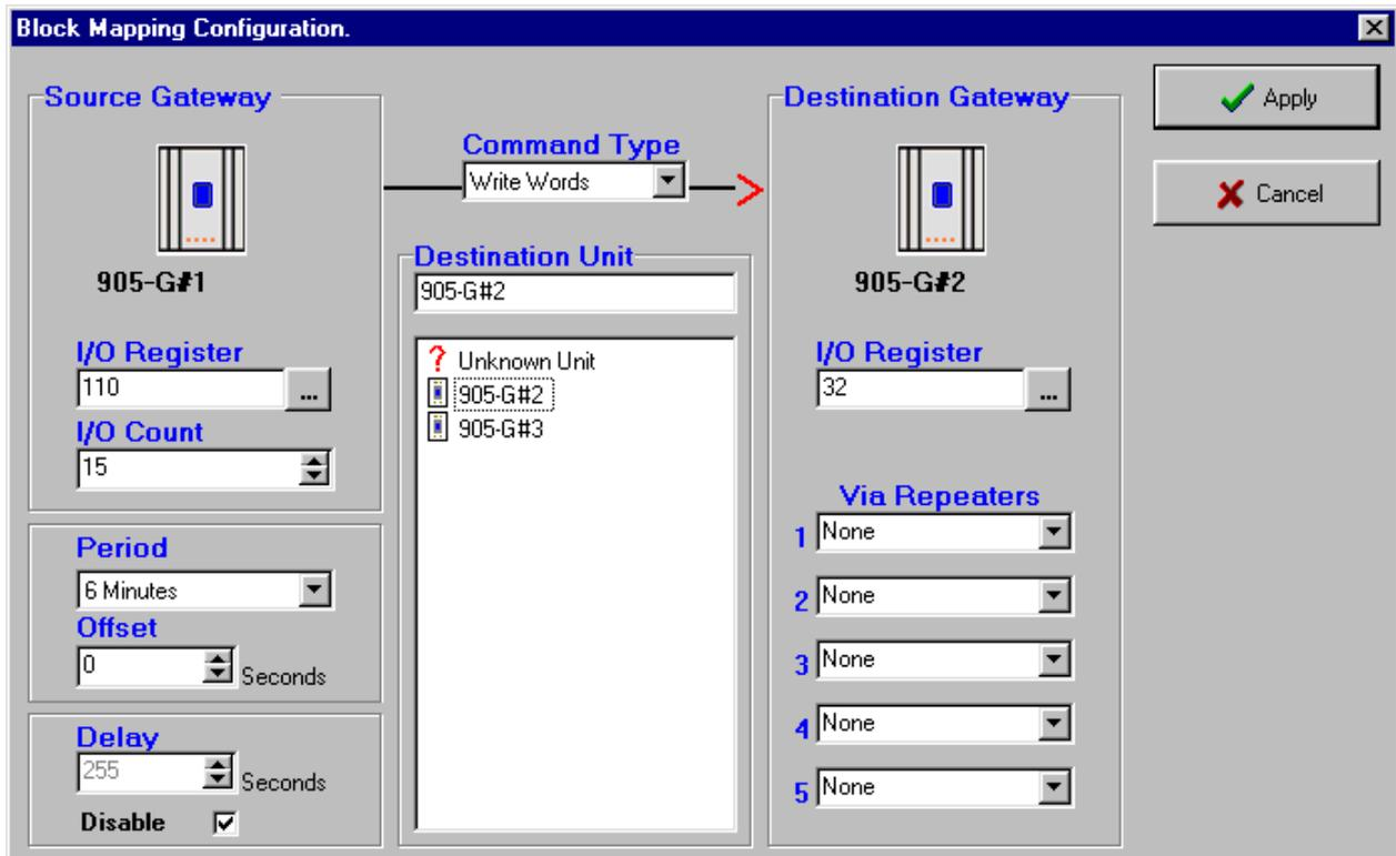
The “Offset” value provides an offset to the specified time. In this example, if the “Offset” was set to 10 seconds, then the messages will be sent 10 seconds later - at XX:00:10, XX:06:10, XX:12:10 etc.
