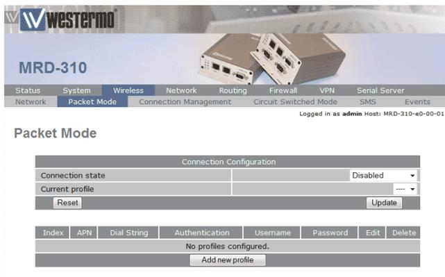
The 3G network provider will provide the items listed below which should be entered into the appropriate fields in the "Add new profile" section as shown in figure 10.
