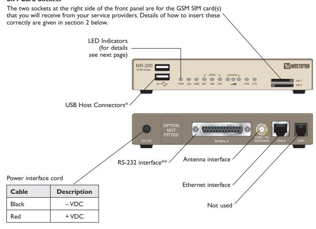
\* The USB host connectors may be used to connect compatible USB 2.0 client devices such as memory sticks, serial adapters, etc. Note that the total current available to power USB devices is collectively 0.5A (i.e. for both ports).
