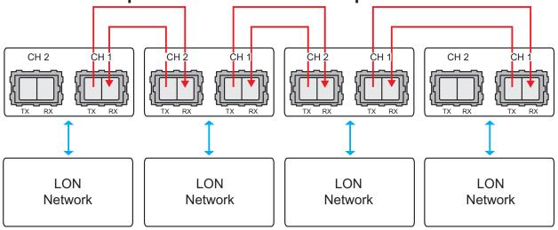
The data is transferred via the fibre optic network to the serial ports of all units. If LRW-112 is connected to two optical fibre links (mid unit) converted data will be transmitted in both directions, via both CH 1 and CH 2. With only one optical fibre link (end unit) converted data will be transmitted in one direction, via CH 1 only. Data received from one LRW-112 optical fibre port will be repeated through the other optical fibre port and it will also convert the frame to serial data.
