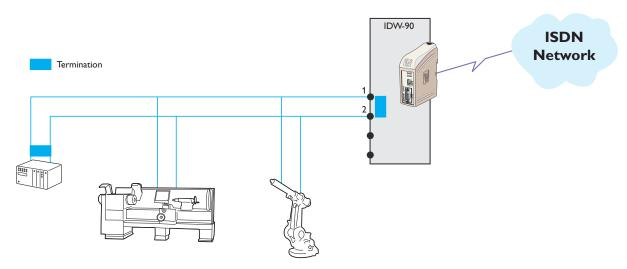
In this application the IDW-90 is set to communicate with a number of units with RS-485 interface. The communication is 2 wire half duplex at 38 400 bit/s, 8 data, parity even and 1 stop bit.
