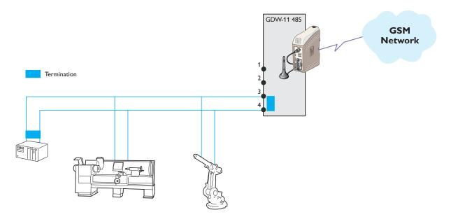
In this application the GDW-11 485 is set to communicate with a number of units with RS-485 interface. The communication is 2 wire half duplex at 38 400 bit/s.
