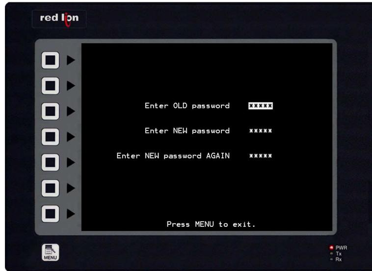
The Change Password page allows you to enter a new password to prevent access to the setup menus. After entering the current password (default password is “0”), you may enter a new one. You must enter the new password twice to ensure you know what you typed! Immediately after entering the new password for a second time, the display returns to the main page.
