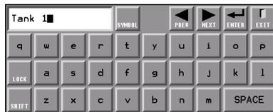
To adjust an alphanumeric field, such as a tank name, simply touch the field, and a keyboard will appear. The keyboard works in a similar fashion to that of a typewriter keyboard, in that SHIFT invokes uppercase for a single character, and LOCK causes the uppercase characters to remain on until you press LOCK for a second time. Pressing SYMBOL, as well as SHIFT+SYMBOL, accesses extra characters such as numeric, punctuation, and symbols.
