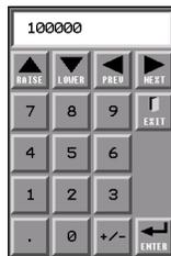
To adjust a numeric field, such as an alarm value, simply touch the field. A numeric keypad will appear, which will allow you to edit the field. Pressing enter will commit the number to memory, and close the keypad.
