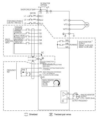
: Only basic insulation (Protective class 1, overvoltage categoly II) is provided for the control circuit terminals. Additional insulation may be necessary in the end product to conform to CE requirements.
