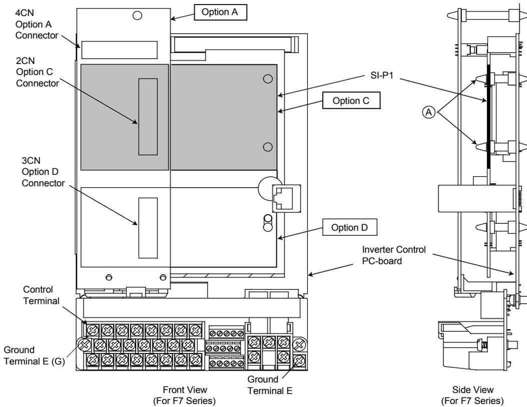
Fig. 2 Installation of PROFIBUS-DP Communications Interface Card SI-P1
