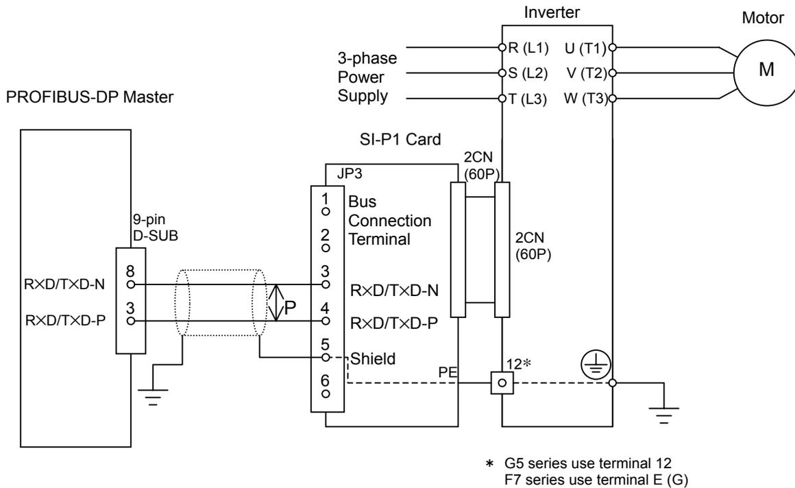
Fig. 3 Interconnection Diagram
