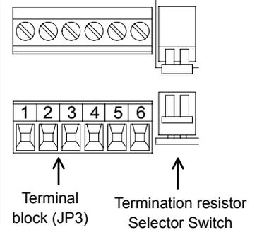
(2) Wire the host PROFIBUS-DP master and SI-P1 card on the terminal block as follows;
