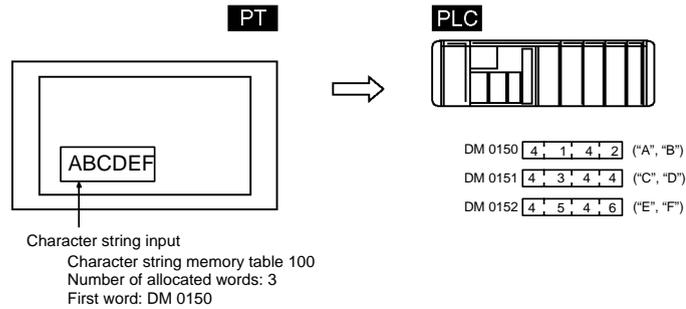
Allocate character string tables to any desired words in the PC. When text is input with a character string input, the new character string will be written to the character string memory table and the contents of the words allocated in the PC will be changed automatically. This function allows text to be written from the PT to the PC easily.
