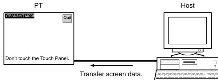
**Reference:** Do not touch the touch panel while screen data is being transferred by the memory link online transfer function. (Do not press the Exit touch switch either.)
