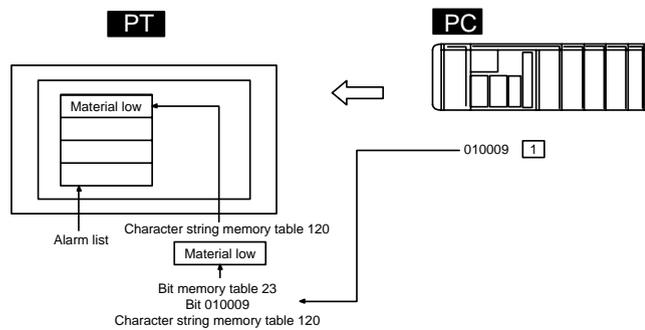
When the PC bit comes ON (1), the contents of the character string memory tables registered for the bit memory tables are displayed in the alarm list. When the bit returns to the OFF (0) status, the character string memory table display is automatically cleared.
