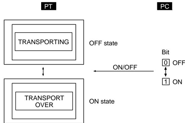
Register a normal lamp for the screen with the following settings.
