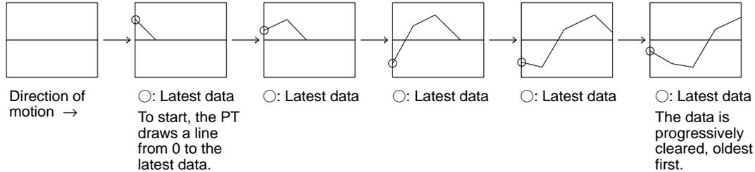
The drawing results with each Direction setting are indicated below.
