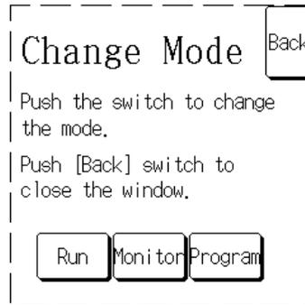
2. Press the touch switch of the desired operating mode. The PC's operating mode will be switched to the specified mode and the operating mode displayed in the bottom-right corner will also change.
