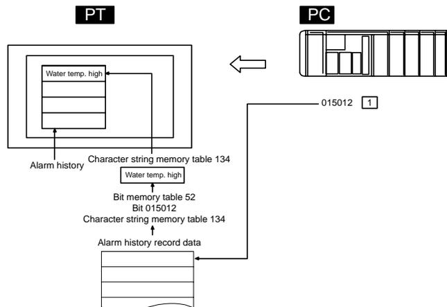
The PC bit allocated to bit memory table for which the history property has been set is continually monitored: when the bit comes ON (1), the time and the number of times, and the contents of the character string memory table registered for the bit memory table, are recorded in the alarm history record data.
