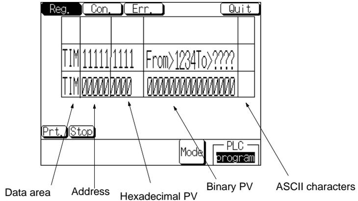
With the NT31/NT31C, the PVs of up to 3 words can be displayed simultaneously.
