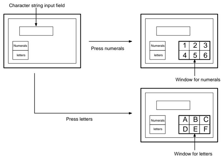
**Reference:** In order to make numeral/character string settings, a key to confirm the input numeric value or character string is required. Allocate the ENT input key-control or Enter (
