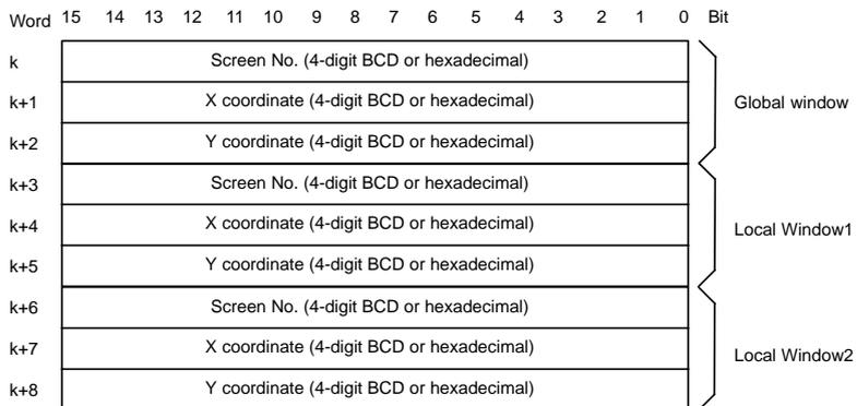
With the program in the host, read out window screen number, X coordinate and Y coordinate in a window control area which corresponds to the window of which display status is to be checked.
