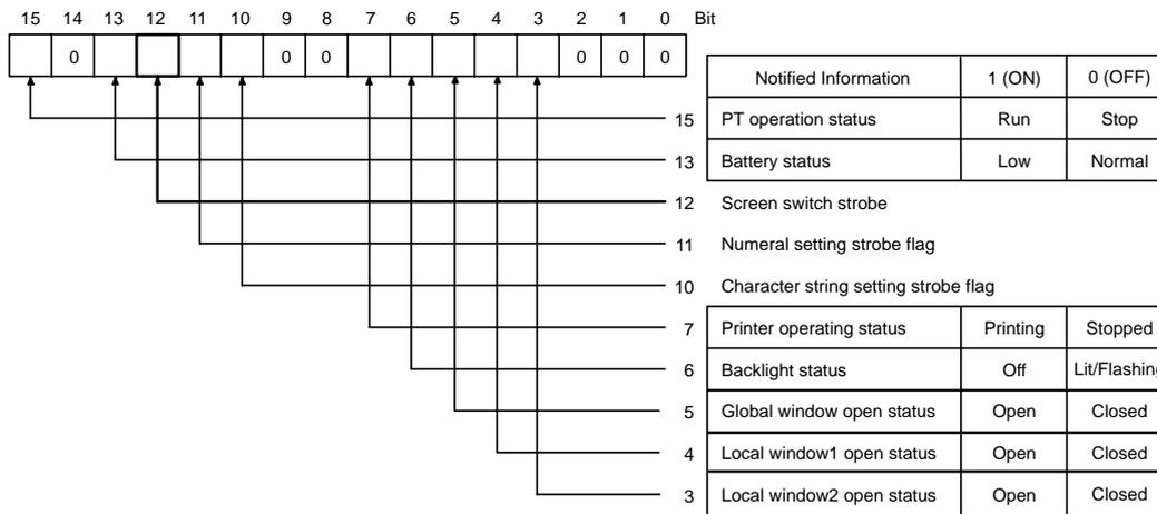
Make a program which runs in the host so that leading edge of bit 12 (screen switching strobe) in the second word (word m + 1) from the beginning of the PT status notify area is checked.
