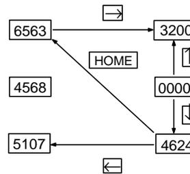
Pressing the HOME key selects the field at the upper left of the screen as the objective input field. If several input fields are arranged at the same distance from the upper left corner of the screen, the one at the left most position is selected as the objective input field.
