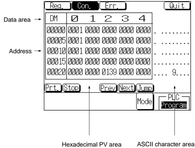
With the NT31/NT31C, the PVs of up to 25 words (5 words × 5 rows) can be displayed simultaneously.
