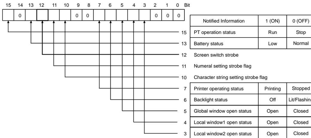
To check the operating status of the printer, operate the PT status notify area in the manner shown below.
