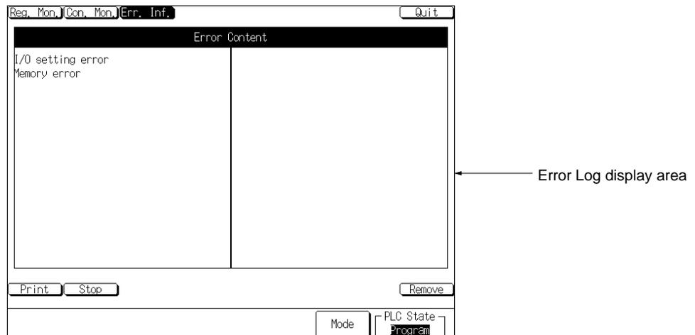
With the NT631/NT631C, 30 error records (15 records × 2 columns) can be displayed in one screen. The highest priority error must be cleared in order to display the thirty-first error record.
