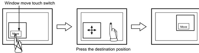
**Reference:** When a window control area is allocated to a host, the bottom left coordinate of the window after moving operation is notified to the window control area. (Refer to page 303)
