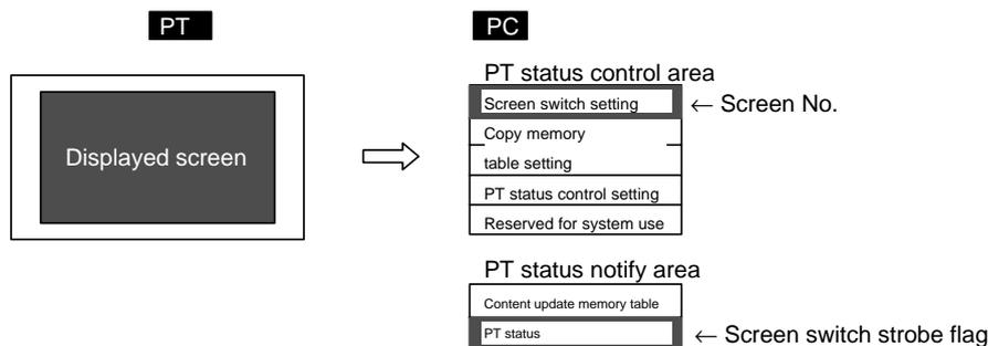
**Reference:** When NT30/620 compatible mode is being used, the current screen number occupies the first word of the PT status notify area and the word containing the PT status notify bits is shifted down one word. (Refer to page 441.)
