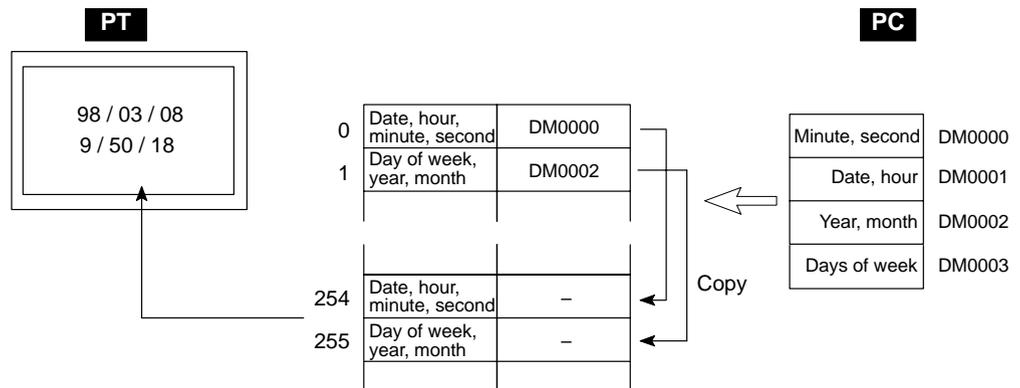
To copy a memory table, either use the PT status control area or the touch switch copy setting function. Here, the procedure for copying a memory table using the PT status control area is described. For the procedure for using the touch switch copy setting function, refer to *Changing Numeric Values/Character Strings by Pressing a Touch Switch Which Has the Copy Setting Function* (page 315).
