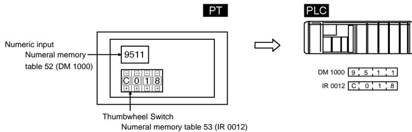
Allocate numeral memory tables to any desired words in the PC. When a value is input or changed with the numeric input or thumbwheel switch, the new value will be written to the numeral memory table and the contents of the words allocated in the PC will be changed automatically. This function allows word PVs to be changed easily from the PT.
