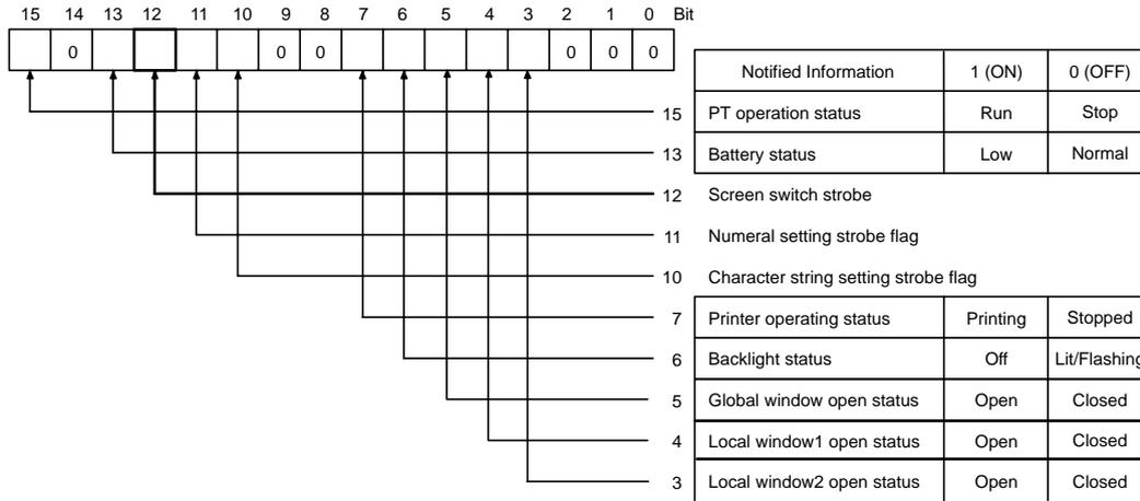
Check the bits from 3 to 5 of the second word (word m + 1) from the beginning of the PT status notify area with the program in the host.
