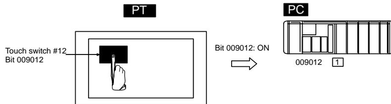
The lamp comes on (flashes) when the PC's bit (lamp bit) is ON (1) and goes OFF when it is OFF (0). When the touch switch is pressed, the PC's notification bit comes ON (1) or goes OFF (0).
