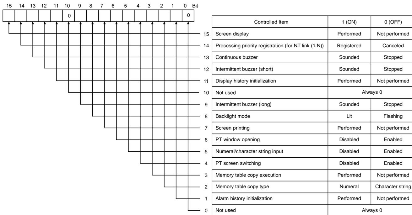
Bits 2 and 3 are not used when the PT is in NT30/620 compatible mode.
