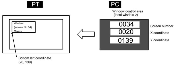
When the window display status changes, the change is notified to the window control area as shown below (Window's Opening/Closing status is notified to the PT status notify area as well).
