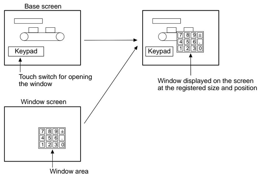
Windows can be called anytime, regardless of which screen is currently displayed. It is possible to display multiple windows (max : 3) on the same screen, and to open, close or move windows by the control from the host.
