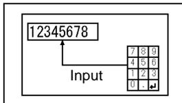
This method uses just an input field. Use the touch switch control keys as a decimal keypad and input values just as you would on a calculator.
