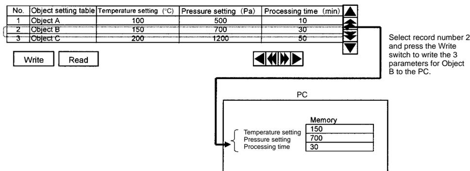
Select record number 2 and press the Write switch to write the 3 parameters for Object B to the PC.
