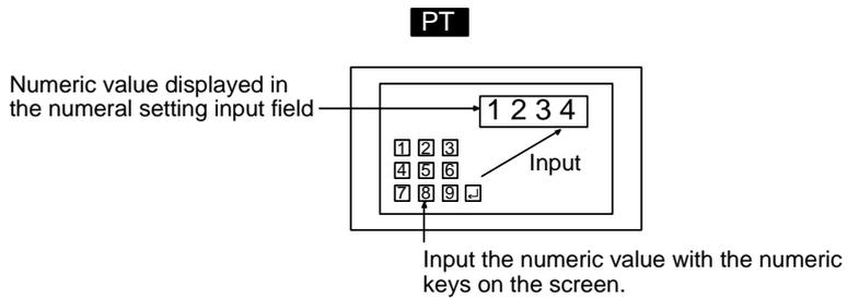
2. On confirming the input numeric value with the ENT key or touch switch it is written to a numeral memory table.
