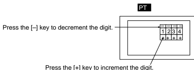
2. Each time a change is made to the numeric value it is confirmed and the occurrence of the change is notified to the host via the PT status notify area.
