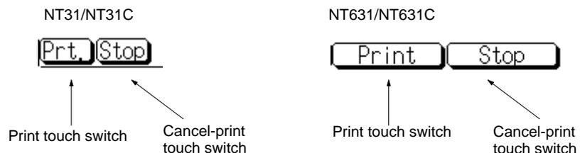
Press the print touch switch to print a copy of the current Device Monitor screen. The screen print can be cancelled by pressing the cancel-print touch switch.
