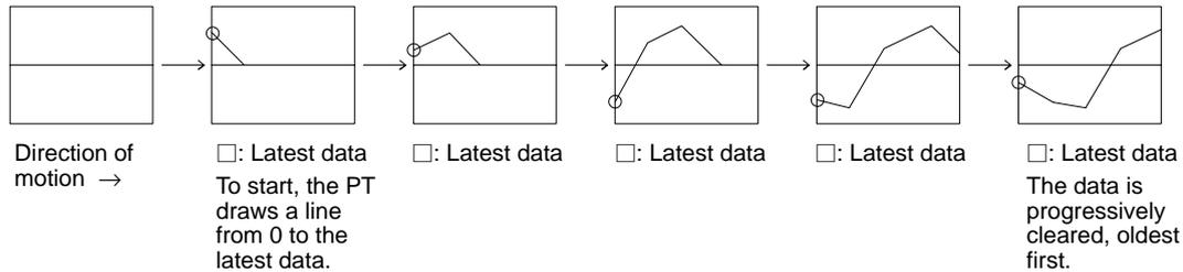
The drawing results with each Direction setting are indicated below.
