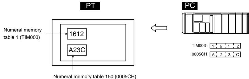
Allocate numeral memory tables to any desired words in the PC. If the contents of the allocated words are changed while the numeral memory table data is being displayed on the screen as numeric values or lamps, the corresponding display on the screen will also change automatically. This function allows the contents of allocated words to be monitored easily.
