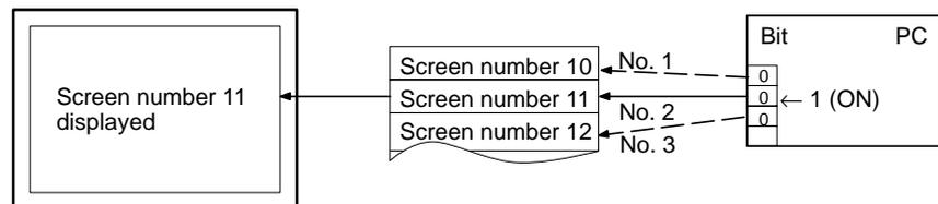
If the allocated bits of multiple bit memory tables come ON at the same time, the bit memory table with the smallest number takes priority.
