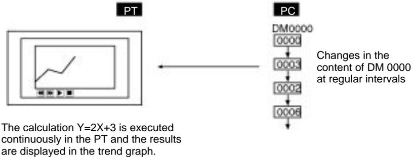
The calculation  $Y=2X+3$  is executed continuously in the PT and the results are displayed in the trend graph.
