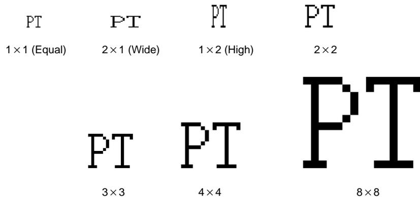
With ISO8859-1 font type, the characters of 2x2 or larger scale are automatically displayed in 32 dot high-definition font. However, the marks inserted into a string are always displayed in 16x16 dot font.
