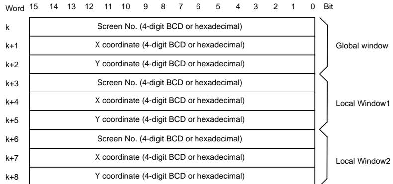
**Reference:** It is not necessary to allocate word to window control area when the window is not controlled from the host or when the window is not used.
