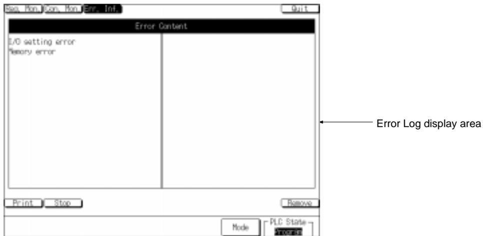
With the NT631/NT631C, 30 error records (15 records × 2 columns) can be displayed in one screen. The highest priority error must be cleared in order to display the thirty-first error record.
