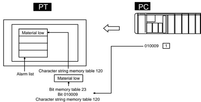
When the PC bit comes ON (1), the contents of the character string memory tables registered for the bit memory tables are displayed in the alarm list. When the bit returns to the OFF (0) status, the character string memory table display is automatically cleared.
