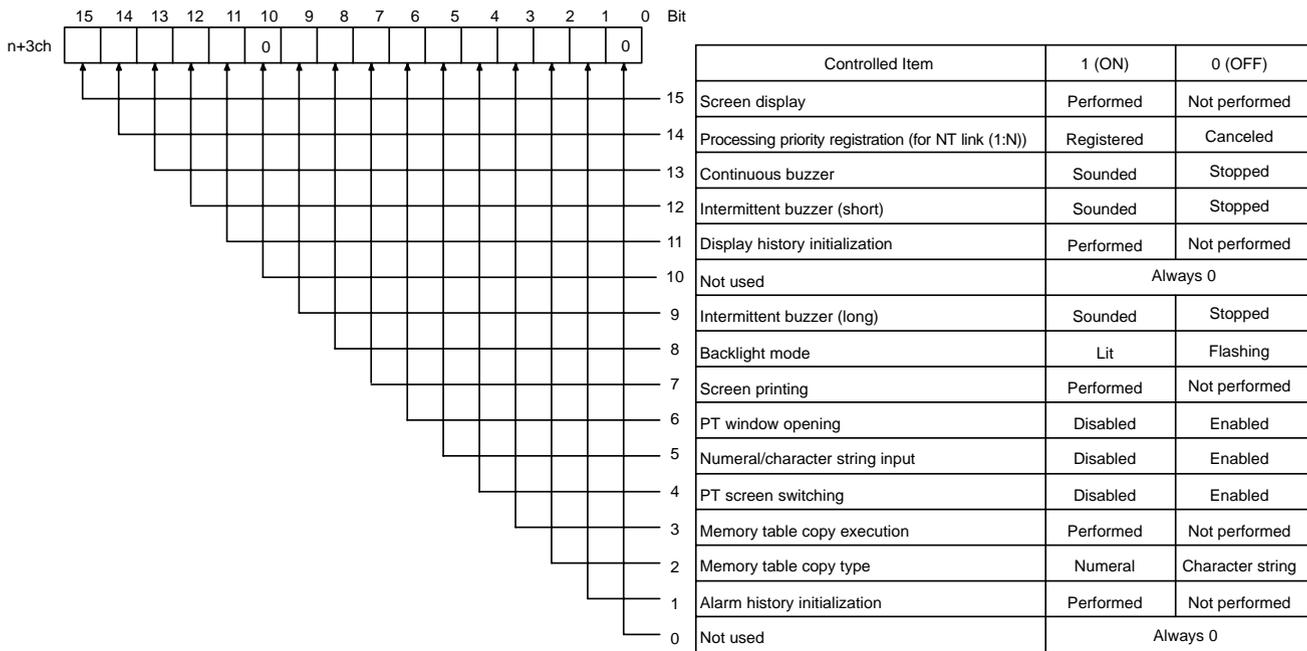
**Note** The backlight mode bit (bit 8) is valid in the NT631.
