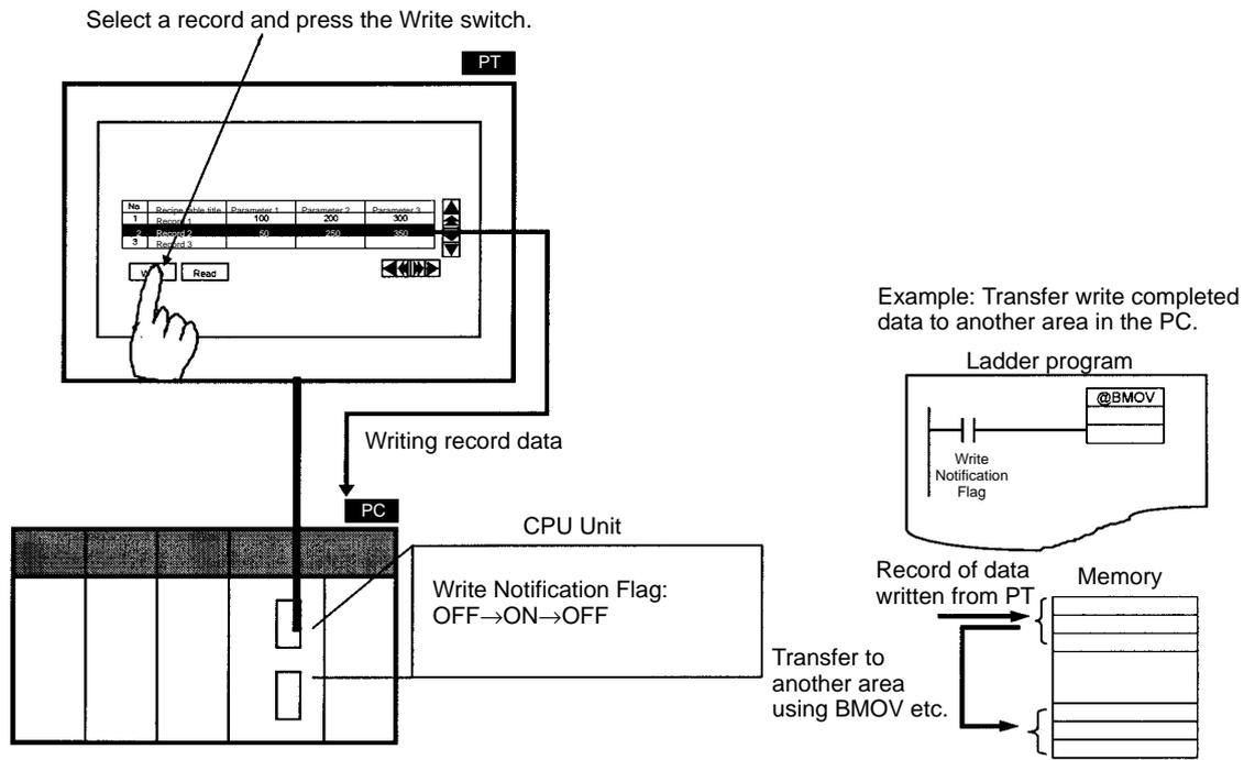
**Reference:** Recipe tables and recipe elements are stored in flash memory within the PT and memory (recipe data memory) that is backed up by a battery. The way that the data is stored is explained below and illustrated in the diagram following.
