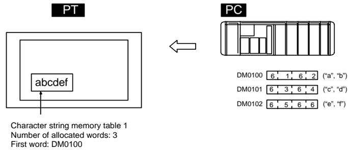
Allocate character string memory tables to any desired words in the PC. If the contents of the allocated words are changed while the character string memory table data is being displayed on the screen as text, the corresponding display on the screen will also change automatically. This function allows any desired message to be displayed easily.
