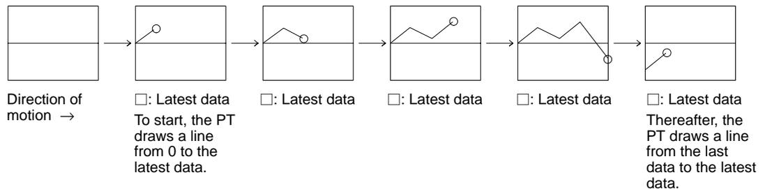
The drawing results with each Direction setting are indicated below.
