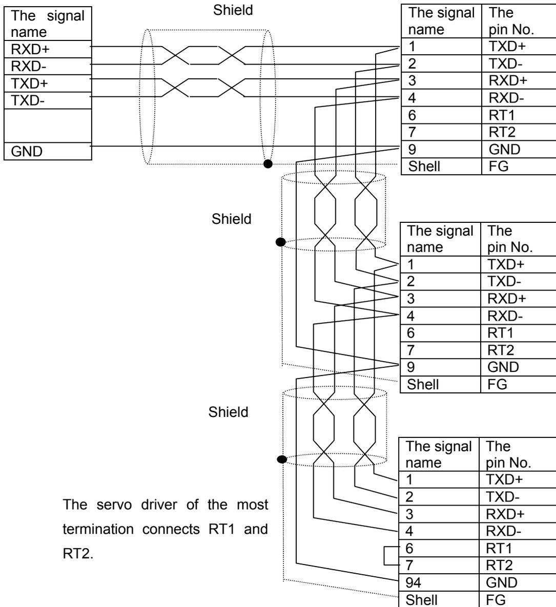
The servo driver of the most termination connects RT1 and RT2.
