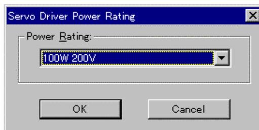
3. It chooses the capacity, the line voltage type of the servo driver to edit from the pull-down menu.
