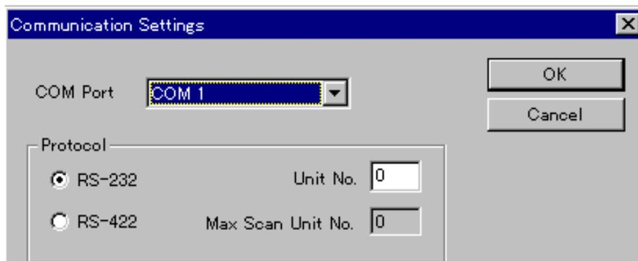
2. It chooses the communication port which communicates with the servo driver by the communication port column.
