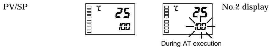
Only the “communications writing”, “run/stop” and “AT execution/cancel” parameters can be changed during AT execution. Other parameters cannot be changed.
