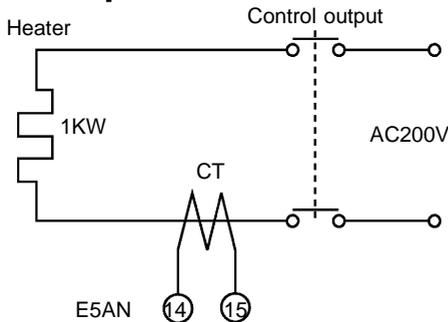
Current during normal operation =  $\frac{1000}{200} = 5\text{A} (< 10\text{A})$
