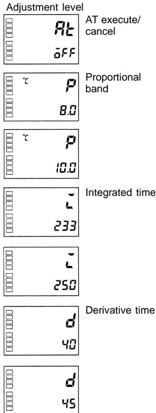
The individual PID constants can be manually set in the “Proportional band”, “integral time”, and “Derivative time” parameters in the “adjustment level”.
