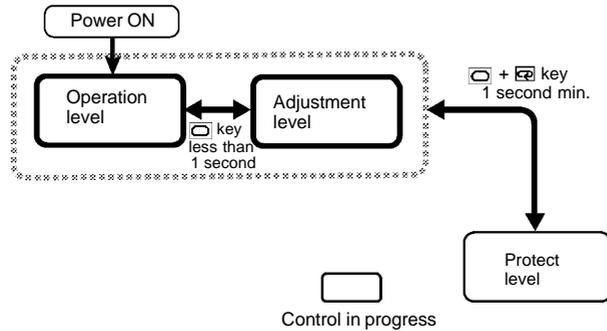
To move from the operation Level to the protect level, press the and keys for at least one second.
