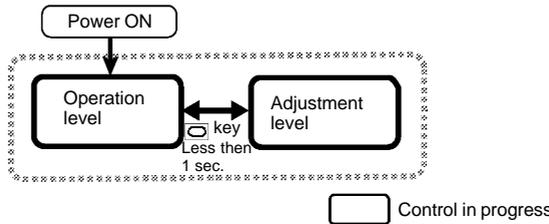
To move to the adjustment level from the operation level, press the key for less than one second.
