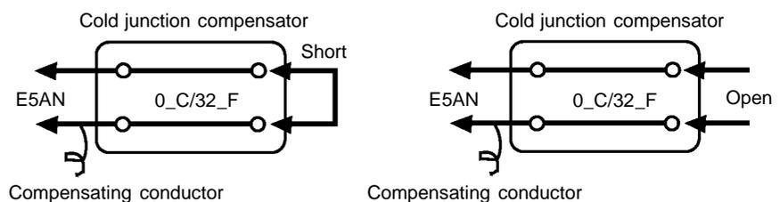
This example describes how to calibrate the E5AN when thermocouple input is currently selected on an E5AN supporting thermocouple input.
