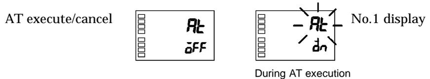
If you move to the “operation level” during AT execution, the No.2 display blinks to indicate that AT is being executed.
