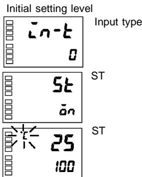
ST (self-tuning) is executed when the “ST” parameter is set to “ON” in the “initial setting level”.
