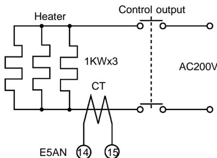
Current at normal operation =  $\frac{1000}{200} \times 3 = 15\text{A} (\geq 10\text{A})$
