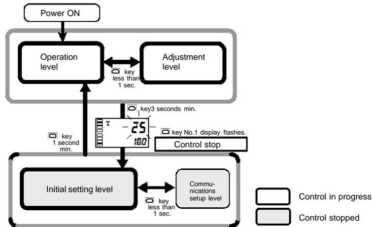
This level is automatically displayed immediately after the E5AN is turned ON. To move to other levels, press the key or the and keys.
