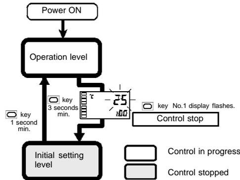
To move from the operation level to the initial setting level, press key for three seconds or more.
