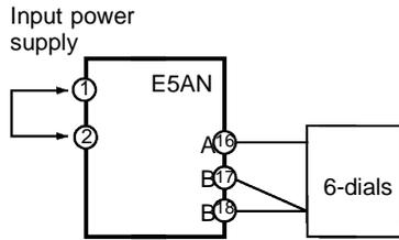
This example describes how to calibrate the E5AN when it is connected to a platinum resistance thermometer.
