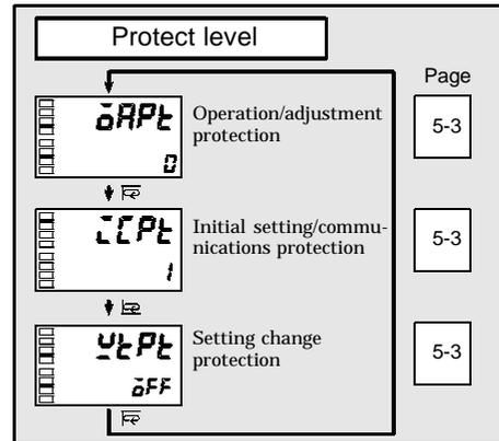
The settings of protected parameters are not displayed and so cannot be modified.
