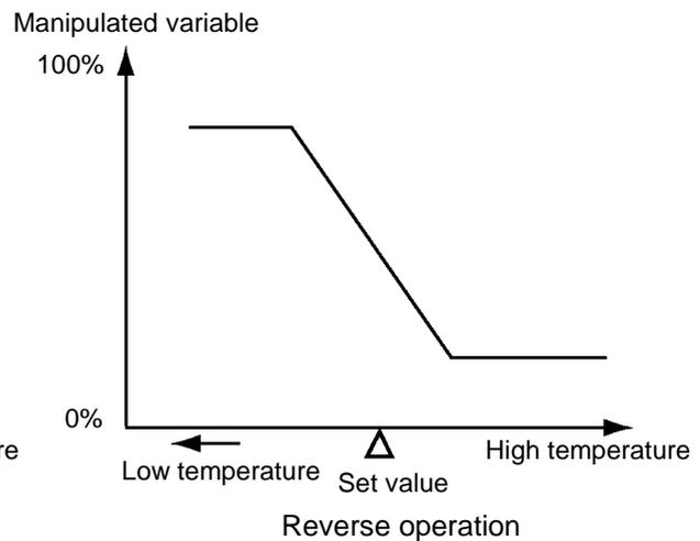
For example, when the process value (PV) (temperature) is lower than the set point (SP) (temperature) in a heating control system, the manipulated variable increases by the difference between the PV and SP values.
