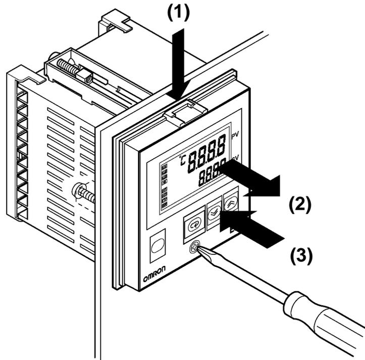
Prepare a screwdriver that can be used on the lower front screw of the unit.
