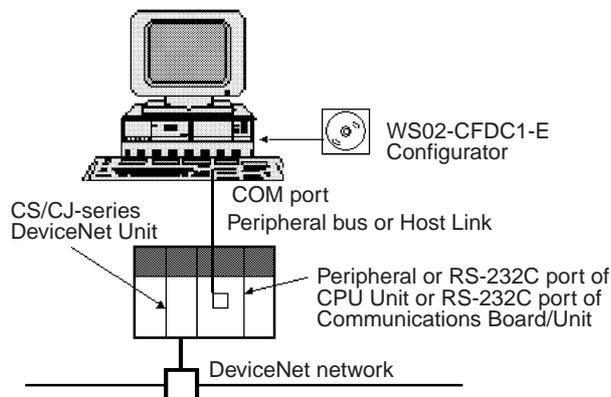
The Configurator is not treated as a single DeviceNet node.
