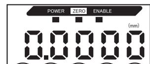
The reference value will be registered and the zero reset indicator will be lit. The tolerance for the registered reference value will be displayed on the main display.
