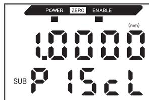
10. Set the sensing object at the position where the display value change is required.
