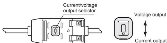
Monitor focus settings are also required when switching the output. p. 95
