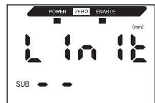
6. Release the ENT Key once OK is displayed on the sub-display.
