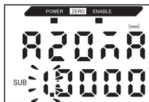
12. Set the output current value and the corresponding measured value for the first point.
