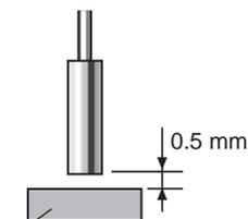
Sensing object: Ferrous object 18 × 18 mm or larger
