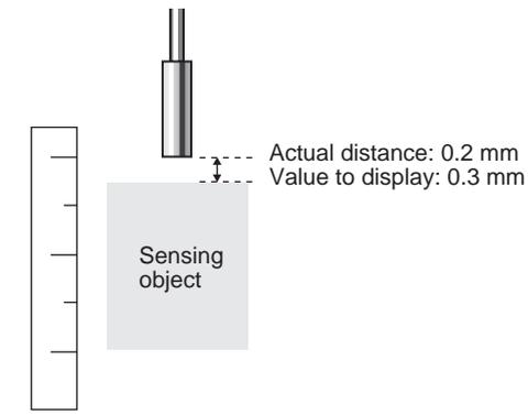
**NOTE** Separate the two specified points by at least 1% of the rated measurement distance for the connected Sensor.
