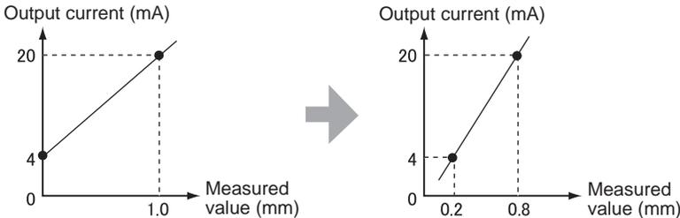
**NOTE** Separate the two specified points by at least 1% of the rated measurement distance for the connected Sensor.
