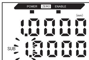
12. Use the Cursor Keys to set the offset for the measured value on the sub-display.
