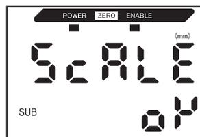
If scaling was unable to be completed, the display will be NG. Check the following points and then execute scaling again.
