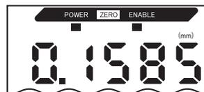
Zero reset will be released and the zero reset indicator will turn OFF.
