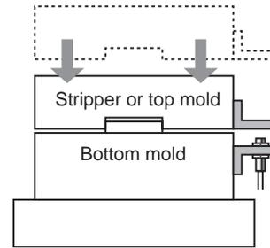
2. Adjust the position of the Sensor Head so that this position is at about half of the measurement distance.
