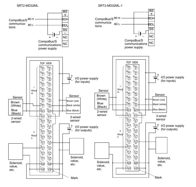
**Note** In accordance with the changes in the standards for photoelectric sensors and proximity sensors, wire colors have been changed. Colors in parentheses are the old wire colors.
