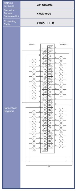
Each V and G terminal is connected internally.
