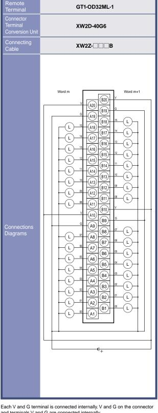
and terminals V and G are connected internally.
