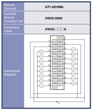
Each V and G terminal is connected internally. V and G on the connector and terminals V and G are connected internally.
