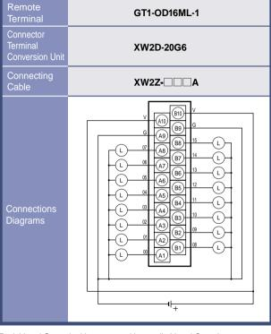
Each V and G terminal is connected internally. V and G on the connector and terminals V and G are connected internally.
