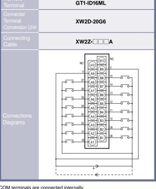
COM terminals are connected internally.
