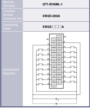
COM terminals are connected internally.
