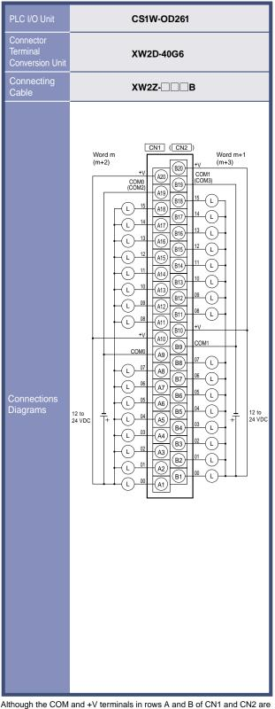
respectively connected internally, wire to all the terminals.
