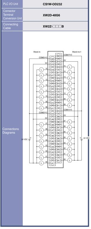
Although the COM(+V) and 0V terminals in rows A and B are respectively connected internally, wire to all the terminals.
