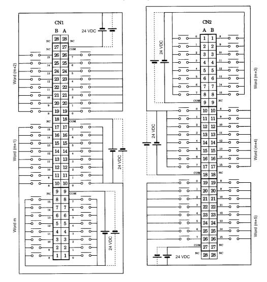
• The polarity of the input power supply can be in either direction, as indicated by the dotted lines.
