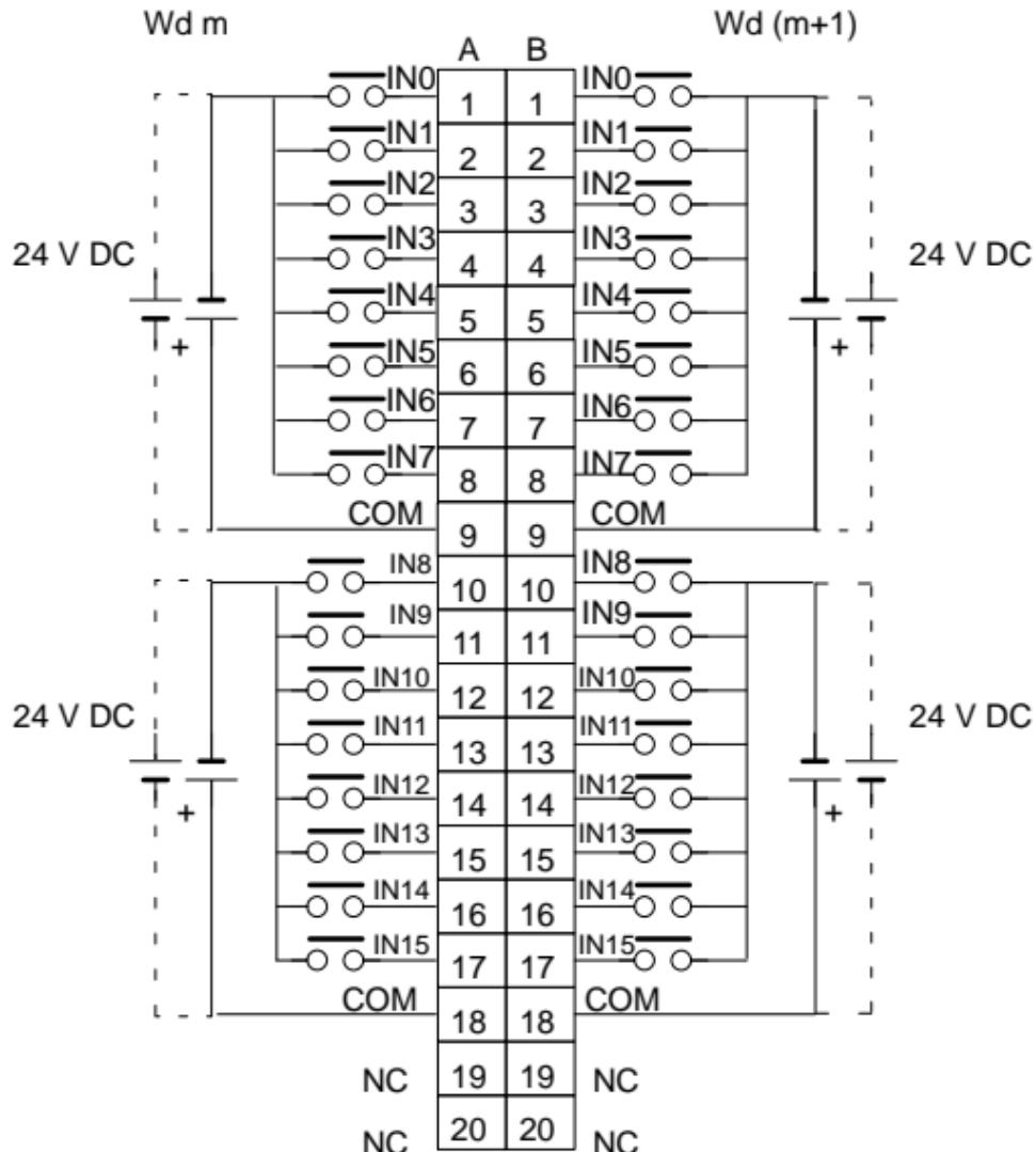
The polarity of the input power supply can be either plus or minus. The polarity of all the commons, however, must be the same. The COM terminals are internally connected, but they all must be wired.
