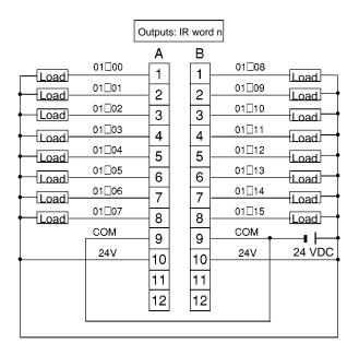
**Note** Wire COM terminals (A9 and B9) and 24-V terminals (A10 and B10) even though they are connected internally.
