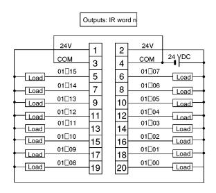
**Note** Wire COM terminals (3 and 4) and 24-V terminals (1 and 2) even though they are connected internally.
