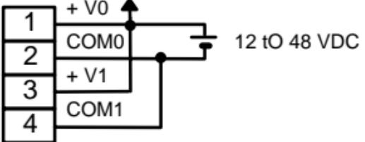
**Note** Select one of the connectors A9, A10, B9, B10, or terminal blocks 1 through 4, and wire them as power and common lines.
