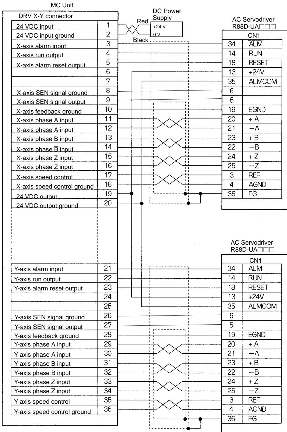
**Note** In the case of the incremental encoder, terminals 5 and 6 on the Servodriver side are connected. However, this can be ignored. Users are not required to connect them.
