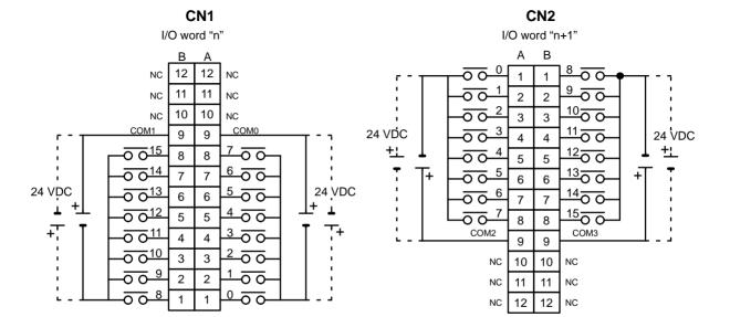
Note 1. When pin 2 of the Unit's DIP switch is ON, input points 08 to 15 in connector 2 are high-speed inputs.
