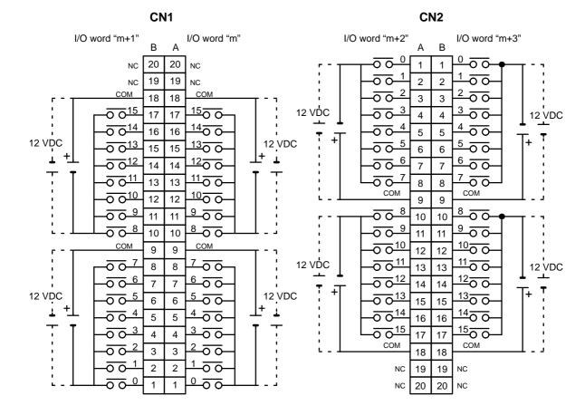
**Note** The power can be supplied in either polarity, but the same polarity must be used for all COM terminals in each connector. Connect power supply wiring to every COM terminal, even though the COM terminals in each connector are connected internally.
