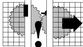
(d1) Check the machine is isolated and stopped whenever the interlocked guard door is open.
