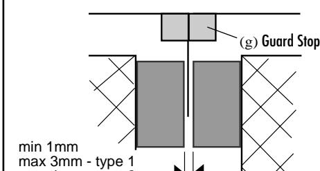
(h) Recommended gap between sensor and actuator.
