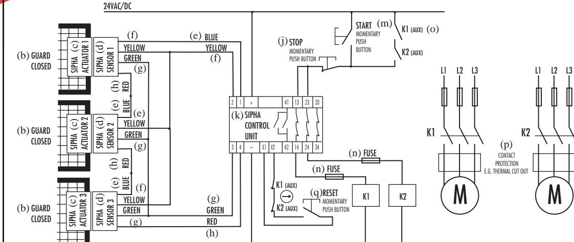
(s) Three sensors and two contactors with manual reset and contactor monitoring. Machine will start when all guards are closed, reset button is pressed and then start button is pressed.
