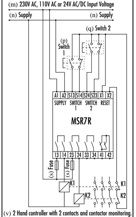
(w) NOTE: Before assuming normal machine operation, check that the outputs are not operated by operating just one of the safety buttons. All outputs must be protected by an external fuse.
