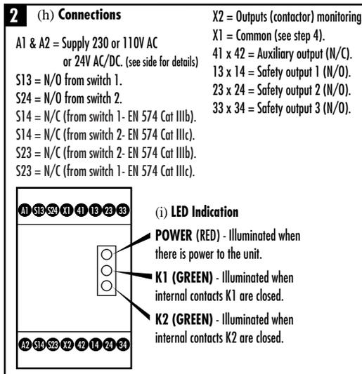
X2 = Outputs (contactor) monitoring.
