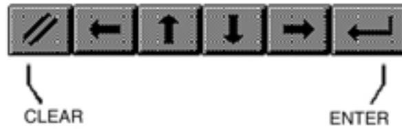
Fig. 26 - Default touch keys for the panels with touchscreen
