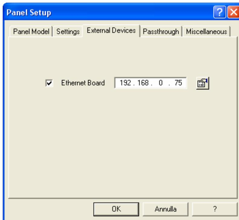
Figure 1 – IP Address in Panel Setup
