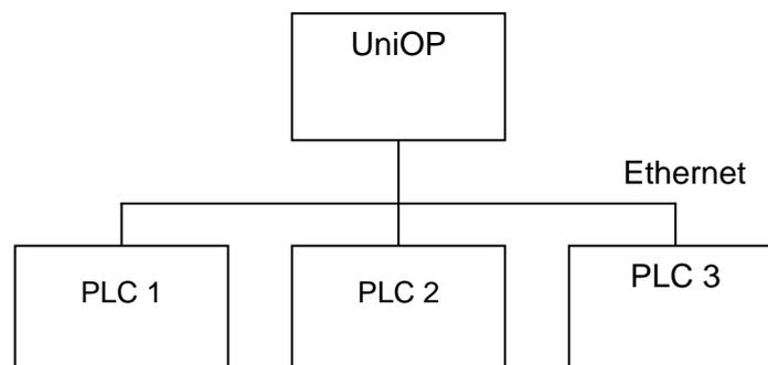
Figure 3– Multiple Controller Connection
