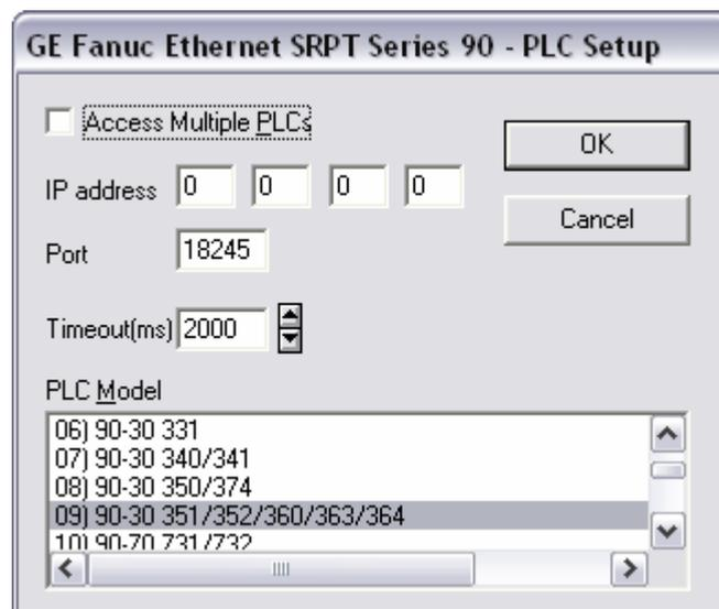
Figure 1– Controller Setup dialog box
