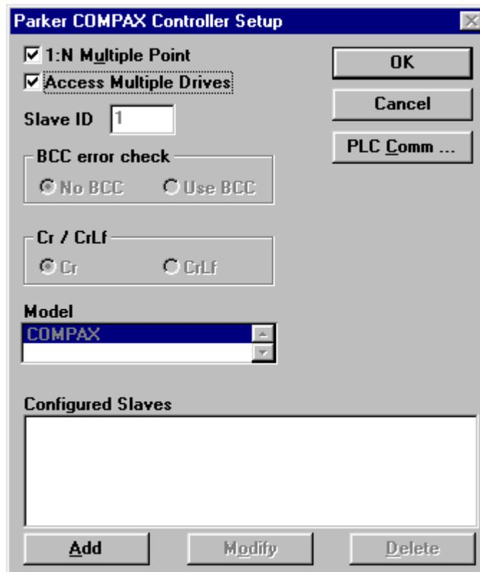
Figure 2 – Controller Setup Dialog Box for multiple controllers setup
