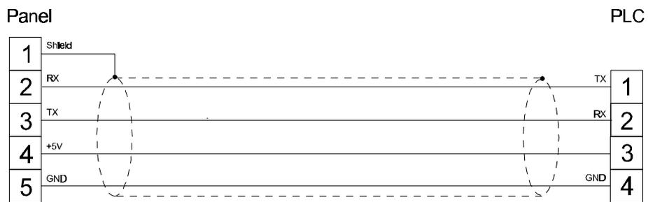
figure 1. Cable diagram
