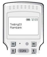
If no errors are detected during the running of the test, the Formula terminal is able to interpret the application commands created with EasyGen<sup>™</sup> and the display screen shows what is indicated in the figure.
