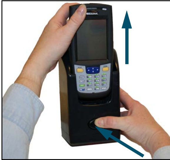
Figure 11. Removing the Pegaso from the Dock
