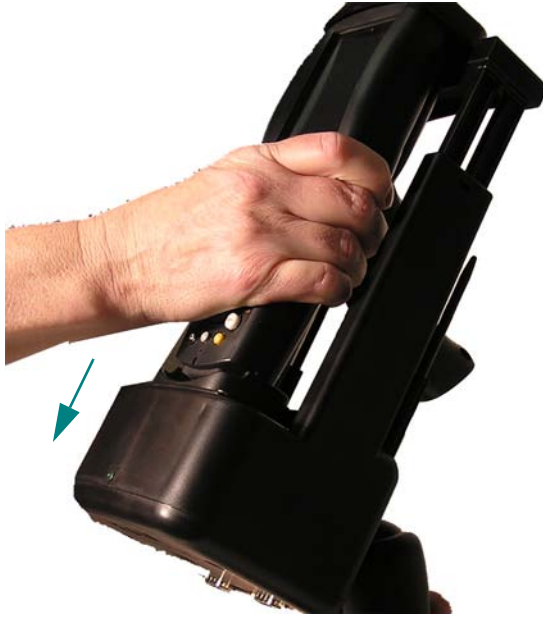
Figure 12. Seating the Falcon into the Dock
