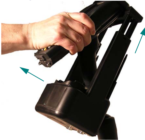
Figure 13. Removing the 4400 from the Dock
