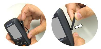
2. Insert the card with the written part upward and push it in, aided by the back of the stylus, until it clicks into place.
