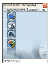
The "Serial Port" button starts communication through the Bluetooth  $^{\otimes}$  serial port COM 5 (typically used for connection with GPS devices).
