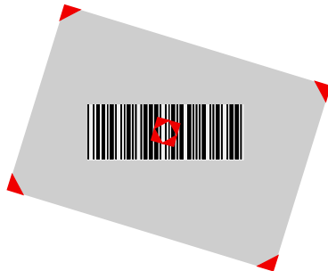
Relative Size and Location of Aiming System Pattern
