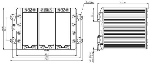
Dimension  $175 \times 100 \times 122 \text{ mm } (6.88 \times 3.93 \times 4.80 \text{ in})$
