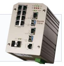
**The MDI-112-F4G** is a 12-port managed Ethernet switch with a flexible port setup including 8 10/100BaseTX ports and 4 10/100/1000 RJ-45/100-FX/Gigabit SX/LX combo ports. The MDI-112-F4G is equipped with advanced ring technology supporting multiple rings, dual homing rings and RSTP as well as a wide range of Layer 2 network features for complex networks such as VLAN, QoS, IGMP Snooping, Port Trunking etc.
