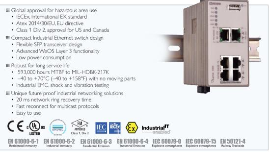
Lynx 206 is a layer 3 managed industrial Ethernet switch, powered by the Westermo WeOS network operating. Independently tested for IECEX and ATEX by Baseefa, as well as Class 1 Division II by FM approval, Lynx is the perfect solution for hazardous area applications in any part of the world.
