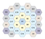
The entire GSM network is organised with cells of varying sizes. A cell can cover areas with a radius of 200 metre (656 ft) up to areas with a radius of  $\sim$ 30 km (18.64 mi). This depends on where the base station is located and the surrounding environment.
