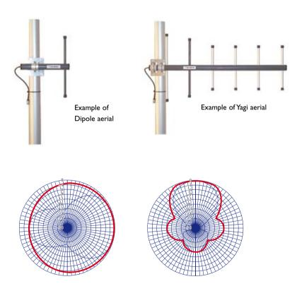
Radiation patterns for omni directional antennas (left; Dipole) and directional antennas (right; Yagi).
