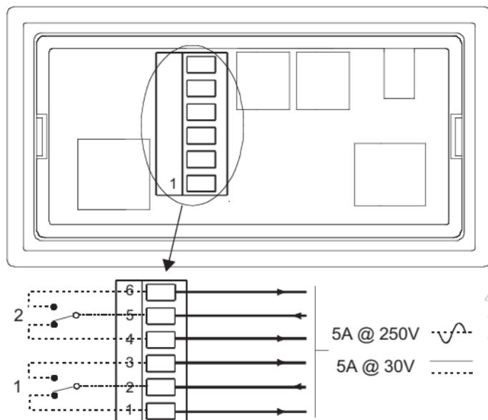
Relays shown in released (not operated) state.
