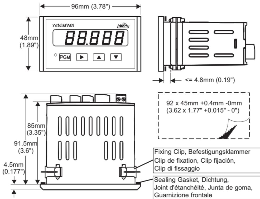
DO NOT OVERTIGHTEN screws, or the gasket will be squeezed out from behind the bezel.
